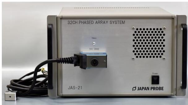
Figure 2: Photograph of 32ch pulser/receiver and array sensor.
