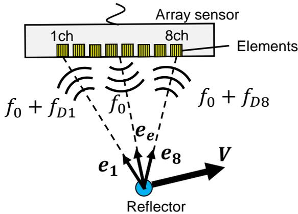
Figure 4: Doppler frequency difference with array configuration.
