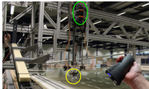
Figure 4: UB-Lab P (within the green circle) installed on the carriage
